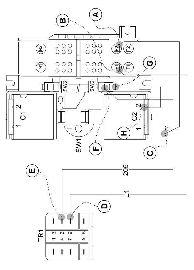
Figure 4. Standby Control Circuit Test Points
